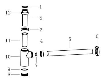
Adjust height of tubes (2) and (11) to required height to meet basin waste and align with main waste pipe, then secure nut (3).
